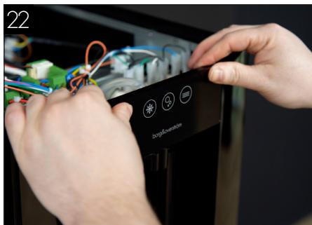
Re-apply the HMI control panel to the front of the dispenser. Press firmly around all edges to ensure a strong bond.
