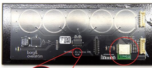
When updating a Version 2 PCB control board with the Firmware Upgrade Key you need the **Number 2 switch in the UP position** and the remaining switches in the DOWN position.
