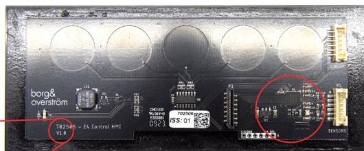
When updating a Version 1 PCB control board with the Firmware Upgrade Key you will need the **Number 1 file select switch in the UP position** and the remaining switches in the DOWN position.
