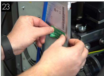
Place the ePTC compressor starter relay upgrade sticker from your pack onto the back of the dispenser, covering up the existing compressor control board sticker.
