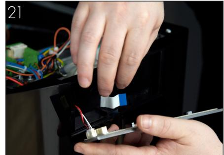
After removing the firmware key, remove the sensor loom and ribbon cable from the touch control board PCB. Push the sensor loom and the ribbon cable back through the slots in the front panel and reconnect them to the HMI control panel. Also reconnect the Sensorbeam® connection, if your dispenser has it.
